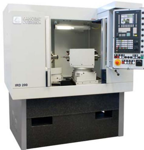
The Danobat-Overbeck IRD-200 grinding machine is ideally suited to the machining of automotive components, dies and short punches.
